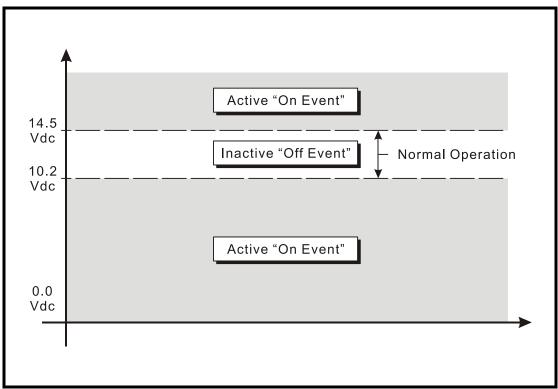
Figure 4 - Analog Input Operating Regions vs. Limit Values
