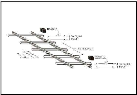
Figure 5 - Typical Installation - Train Speed Monitor
