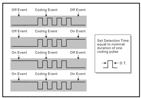
Figure 3 - Typical Code Signal Sequences
