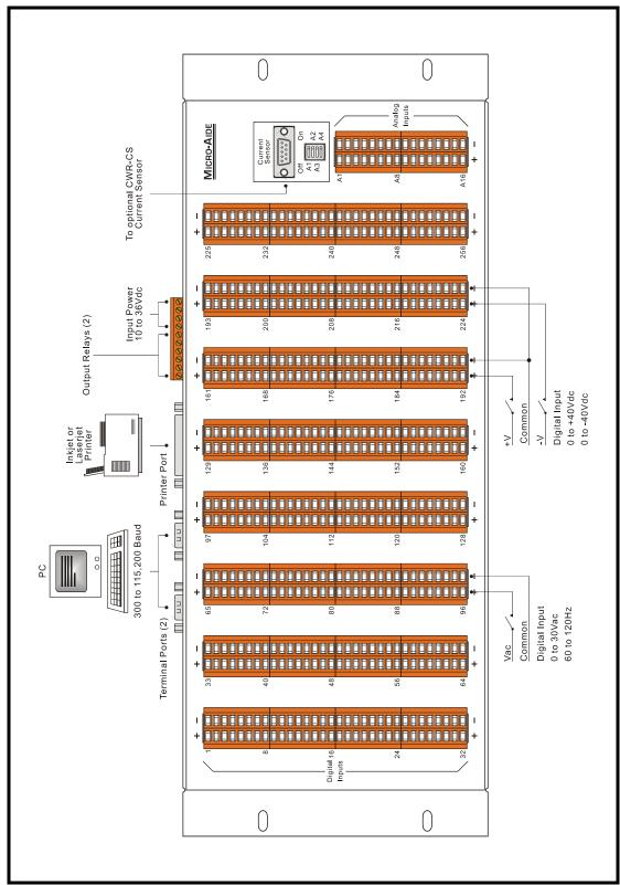
Figure 2 - Typical Installation - Rear Panel View
