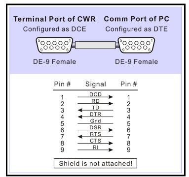
Figure 7 - Terminal Port - Wiring Diagram
