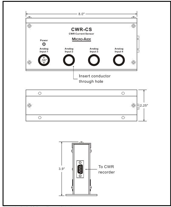
Figure 8 - CWR-CS Front, Top and Side Views
