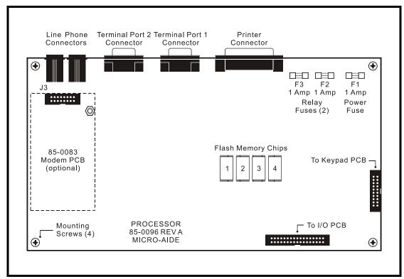
Figure 6 - CWR-272 Processor PCB
