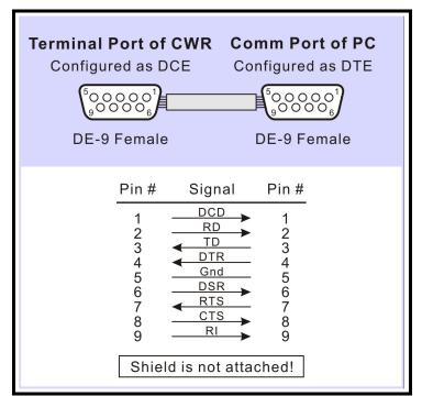
Figure 13 - Terminal Port Cable - Wiring Diagram
