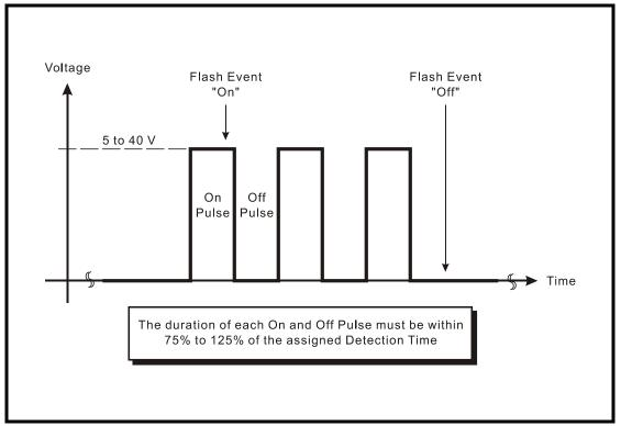
Figure 8 - Typical Flashing Pulse Sequence
