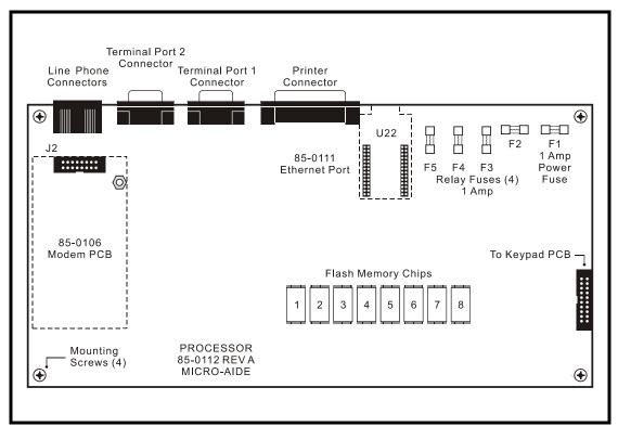
Figure 11 - CWR-264P Processor PCB
