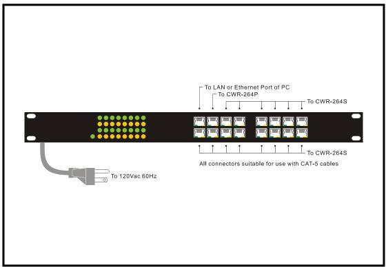
Figure 7 - Typical Installation - 51-0001 Ethernet Switch
