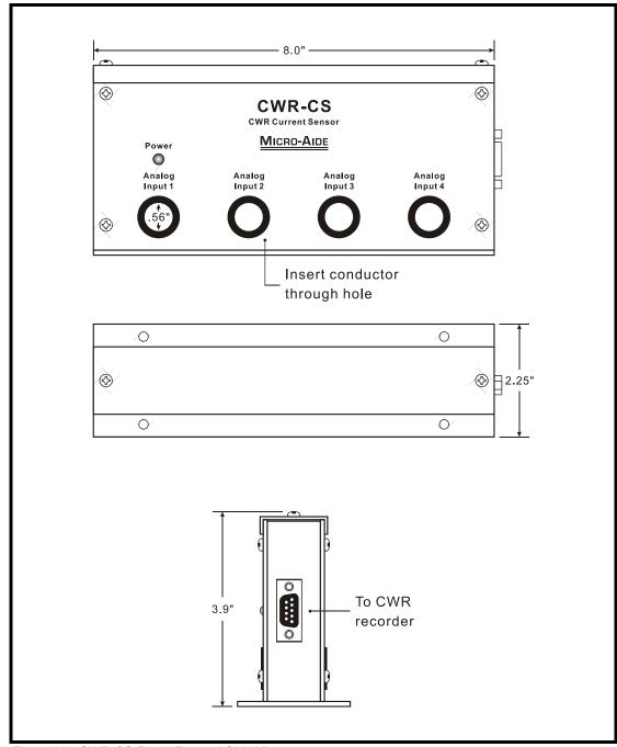
Figure 13 - CWR-CS Front, Top and Side Views
