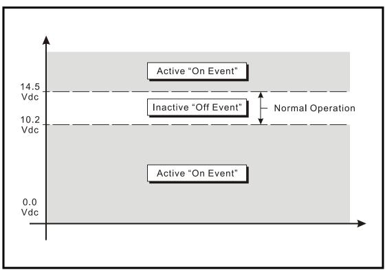
Figure 9 - Analog Input Operating Regions vs. Limit Values
