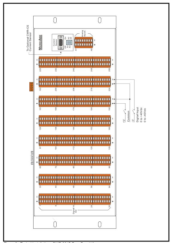
Figure 6 - Typical Installation - CWR-264S Rear Panel View
