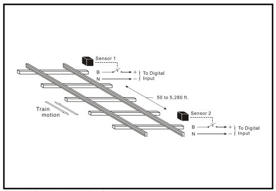
Figure 10 - Typical Installation - Train Speed Monitor
