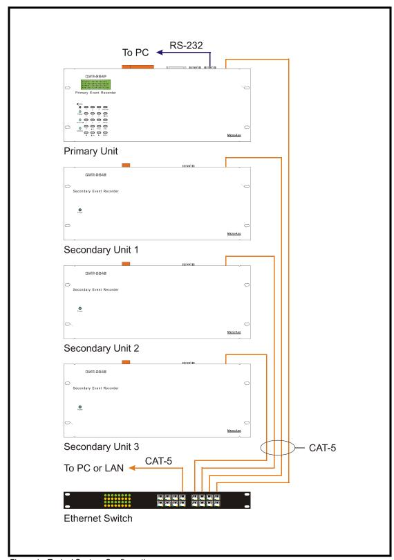
Figure 1 - Typical System Configuration
